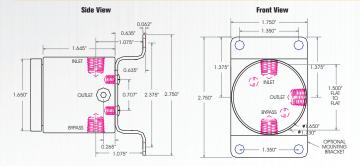
If left outlet required, invert Genie and use port labeled "BYPASS" as inlet, because sample must enter upper port.
