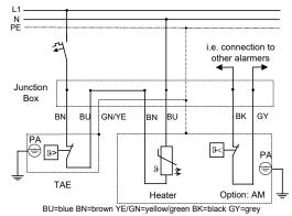
Connection cable Silflex-EWKF 3x1,5 mm<sup>2</sup>, 1m long. Other lengths available upon request (at an extra charge).
